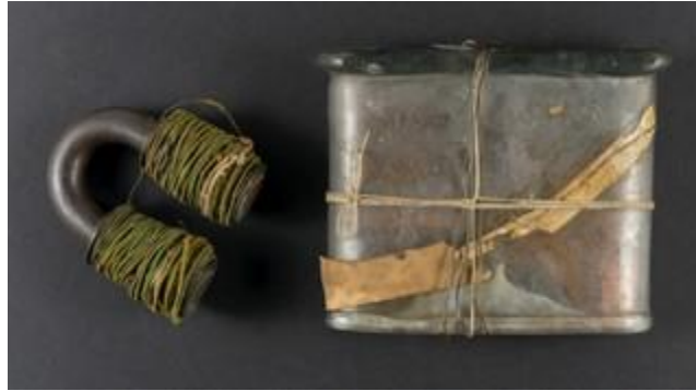
Photo of Hippolyte Pixii's electromagnet.
